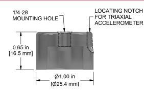
Quick Disconnect Receptacle with 1/4-28 Tapped Mounting Hole
